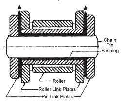
Figure 31. Chain-Link Cross Section
